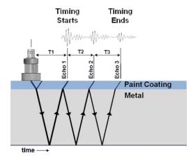
**Single-Echo** uses one back wall echo, measures remaining metal thickness on uncoated surfaces and is possibly helpful for areas with extreme front face or back wall corrosion and pitting. Effective on highly attenuative materials such as cast metals, plastics and composites.
