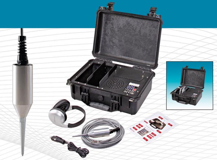
The CDI GeoEAR allows an operator to hear extremely faint sounds at great distances. The GeoEAR can amplify the sound of an approaching pipeline pig's cups striking the welds of a pipe to an easily discernible level, and under normal circumstances a pig can be heard approaching for several miles.
